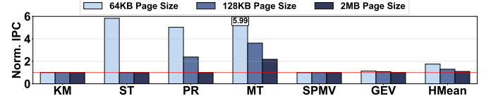
Fig. 20: Speedup of NB-WALKER+AMR over the baseline GPU with varying page size (64 KB, 128 KB and 2 MB).
